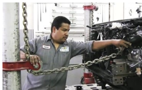
A Campbell Collision Center technician works on a structural straightening job.
